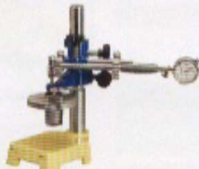
Calibration of Bore Gauge (Horizontal)
