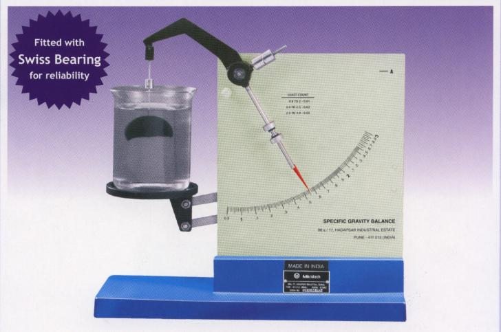
Direct Reading of SPECIFIC GRAVITY for RUBBER AND RUBBER - LIKE MATERIALS
