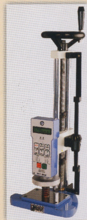
MFG Mounted on Spring Testing Machine
